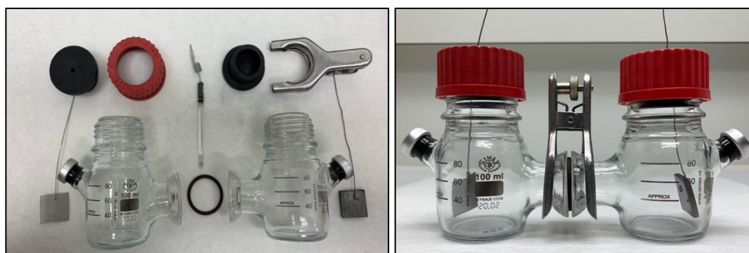
Figure 3.2. Construction of double chamber MECs
